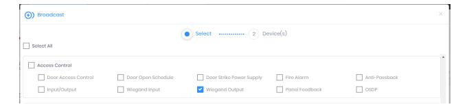
12. Click **Broadcast** and select the rest of the devices in the popup as displayed. Click **OK** to copy all Wiegand output settings of the source device to all destination devices at once.
