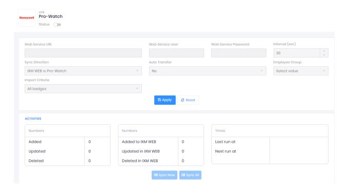
2. Enable editing configuration by toggling the switch next to the logo to **ON**. Data is not synced when the configuration is applied with this switch in the OFF position.
