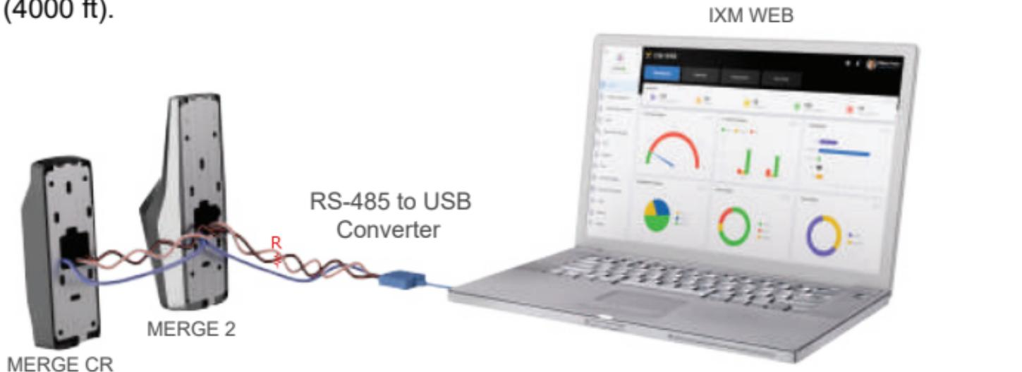
R = 120 ohms for Standard RS-485 Cabling
