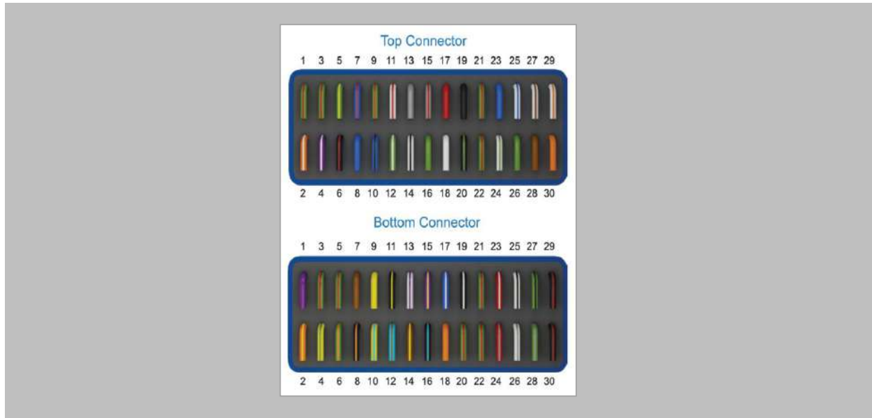
Figure 136: IXM TITAN – Top & Bottom Connector Wiring
